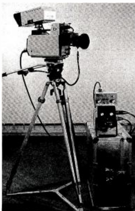
MNC-71CP with 5" viewfinder, mounted on Universal 2030 fluid head tripod (equipped with double handles). Also shown: Remote Production Control Unit and Remote Control Panel ("Palnt Box"), camera case and related accessories.
